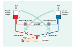
The Single-Needle Cross-Over (SN-CO) name is derived from the control's special feature: When reaching a certain control pressure, the opposite tube clamp closes and the respective other phase begins. Hence, the clamps' control is carried out crosswise: Cross-Over.
