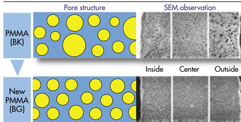
As shown in the figure, BG membrane is designed by homogenizing the pore size and increasing the number of pores, resulting in the improvement of the removal through small molecules to low molecular weight proteins such as  $\beta_2$ -MG.
